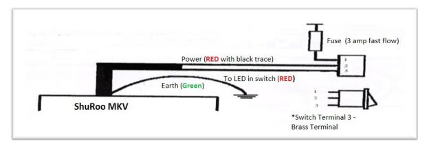
With correct installation, ignition on the dash switch will be activated, ShuRoo will emit a crisp audible "zip zip" sound and the dash light will be steadily illuminated (or flashing) if not illuminated there may be an issue with the wiring or unit.
